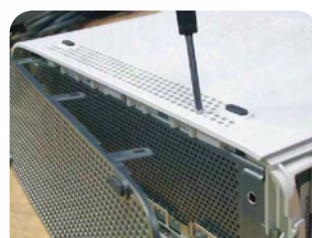
3.Remove the plate holder on top, and remove the front mesh. Repeat the same step for the other side.
