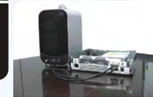
15.After the black industrial grade connectors have been connected, re-assemble all the components, and the Xbox 360 liquid cooling system is complete.
