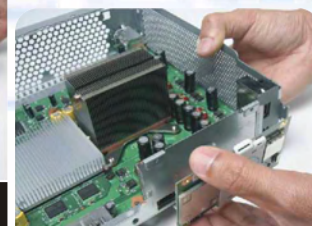
10.Remove the LED indicators.
