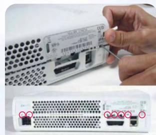
4.Release the 7 tab holders around the unit.
