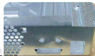
13.On the bottom metal cover, drill two holes. Check to see if they fit the quick connectors.
