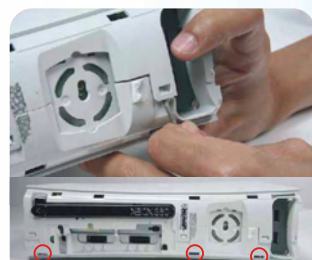
5.Unhook the front tabs and remove the white shell.
