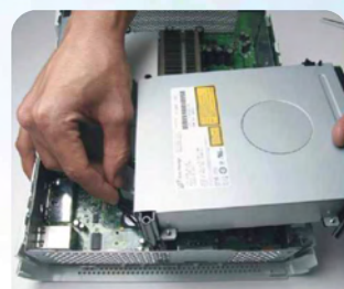
6.Remove the optical drive.
