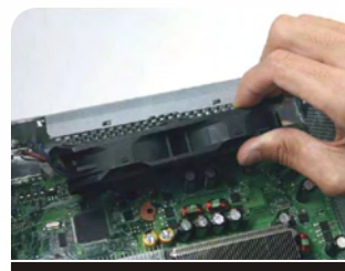
8.Remove the fans as shown.
